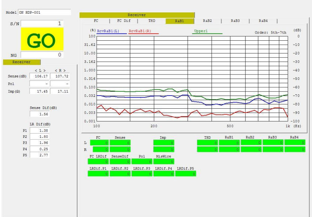
The screen of "Rub and Buzz", Passed the test
