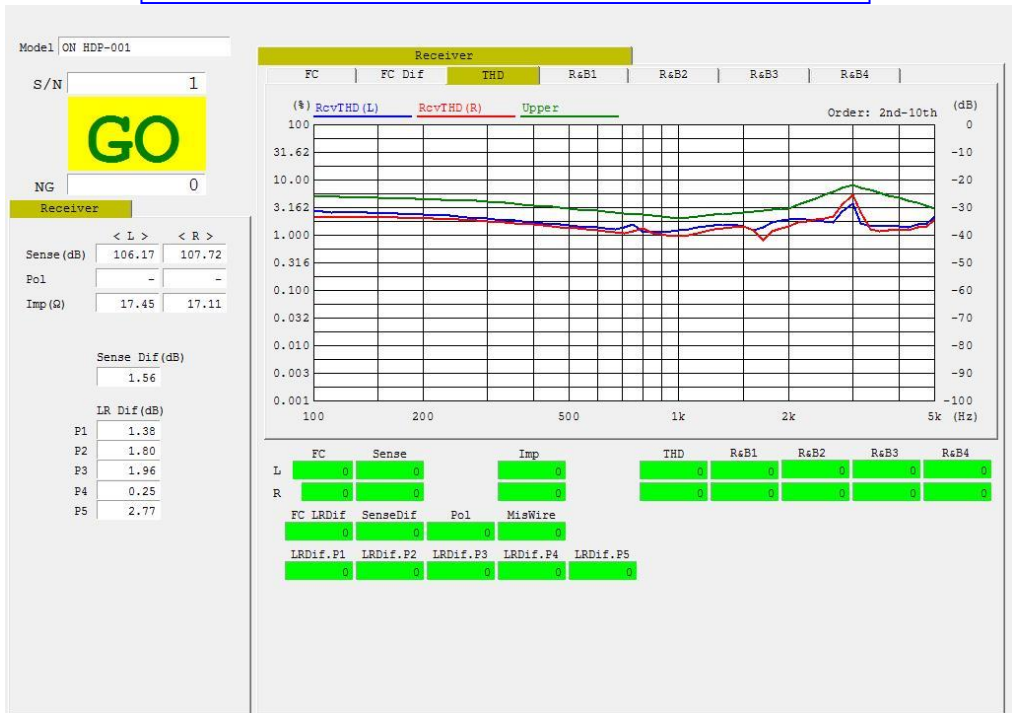
The screen of "Total Harmonic Distortion", Passed the test
