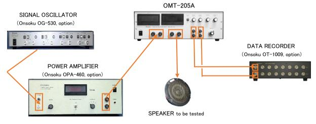
In OMT-205A, the minus terminal is grounded. Therefore when the power amplifier based on "BTL" connection is used, perform the following items.
